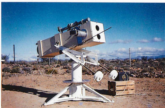
One of the Danjon telescopes, provided in the last stage of the tests with a mask for experiments by A. B. Muller simulating a double beam telescope for measuring image motion. Photograph by D. Beintema, 1962.
