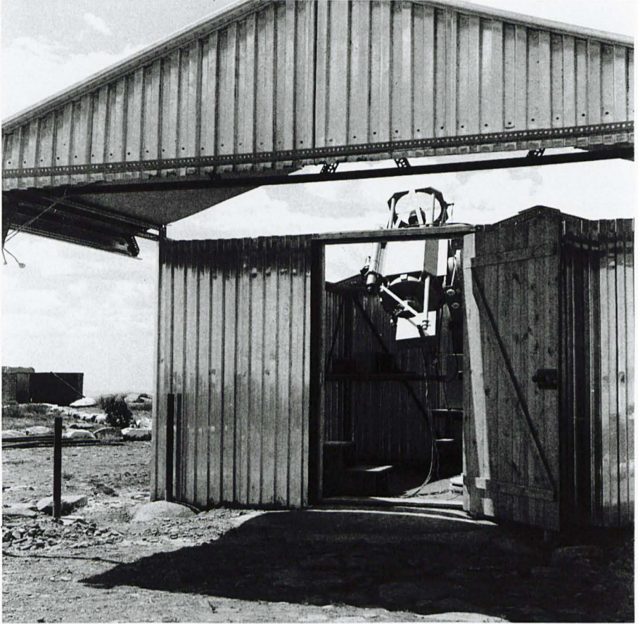
The Tübingen Project. Observers from Tübingen worked on Rockdale Mt. on stellar photometry as well as on the integrated light from the Milky Way. Shown here are the Tübingen 40-cm telescope with photometer in its housing with the roof removed for observing, and in the background at left the wall around the integrated-light photometer.
