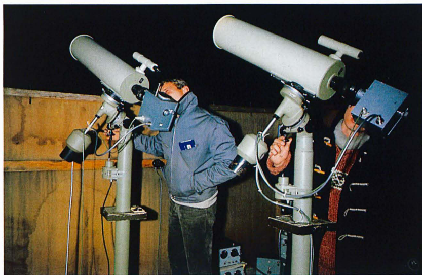
Site testing in the “Comprehensive Program” in 1962. Top: with the Danjon telescope for image quality. Bottom: with photometric telescopes for extinction measures; here: intercomparison check of two telescopes. Photographs by D. Beintema, 1962.
