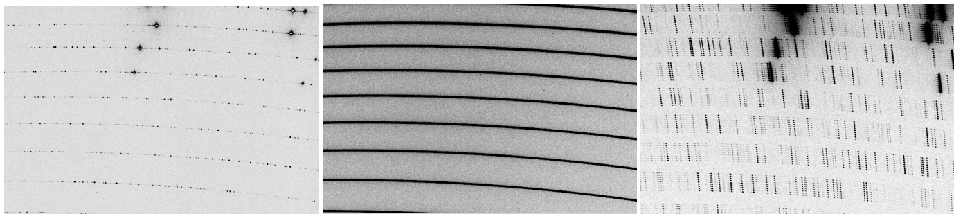
Fig. 7. Sections (1365 pix \times 925 pix) of VIS arm calibration frames used by the data reduction pipeline to fully characterize the spectral format. From left to right: a single pinhole arc frame (“format check”), a single pinhole continuum frame (“order definition”) and a 9-pinhole arc frame used for spatial scale and wavelength calibration.
